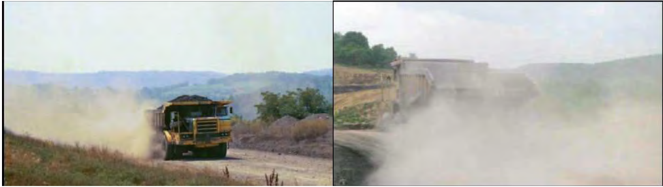
Figure 2: Dust clouds from vehicle travel on unpaved road at a surface mine
