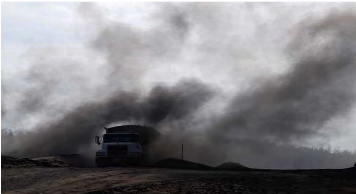
Figure 1: Dust clouds from vehicle travel on unpaved road at CCW landfill in Bokoshe, OK
